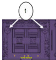
Figure 35: Tighten Screws on the Inserted VIM5 Module
