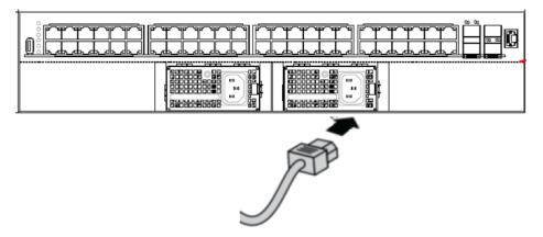
Figure 5: Connecting AC power to the front panel
