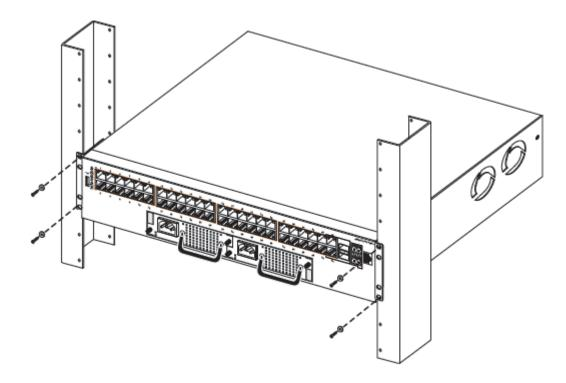
3. Insert and tighten the rack-mount screws.
