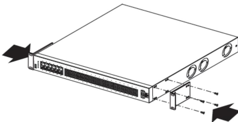
2. Slide the switch into the rack as illustrated.
