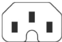
Figure 2: IEC 60320 C16 connector
