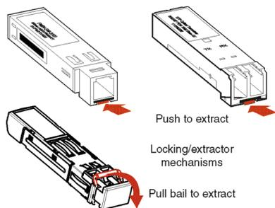
3. Slide the transceiver from the module slot.
