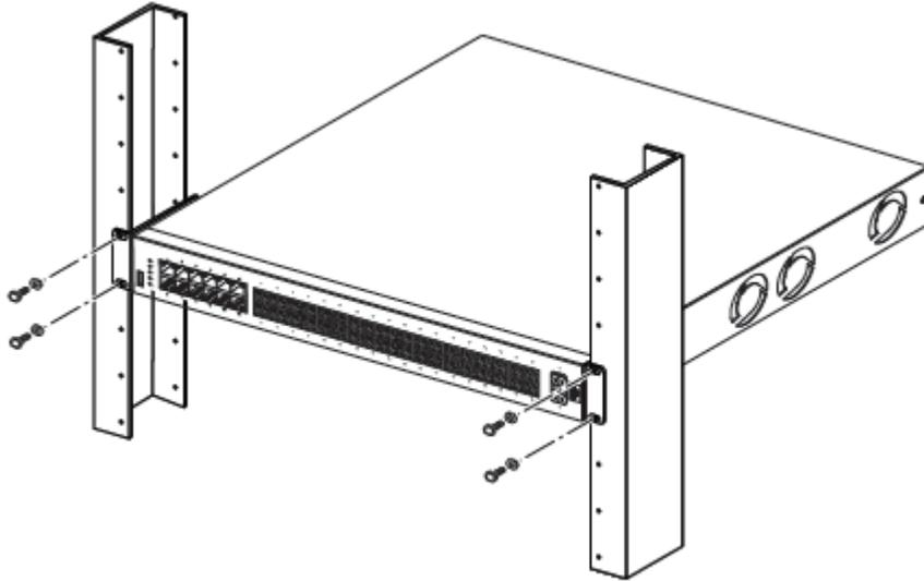
3. Insert and tighten the rack-mount screws.
