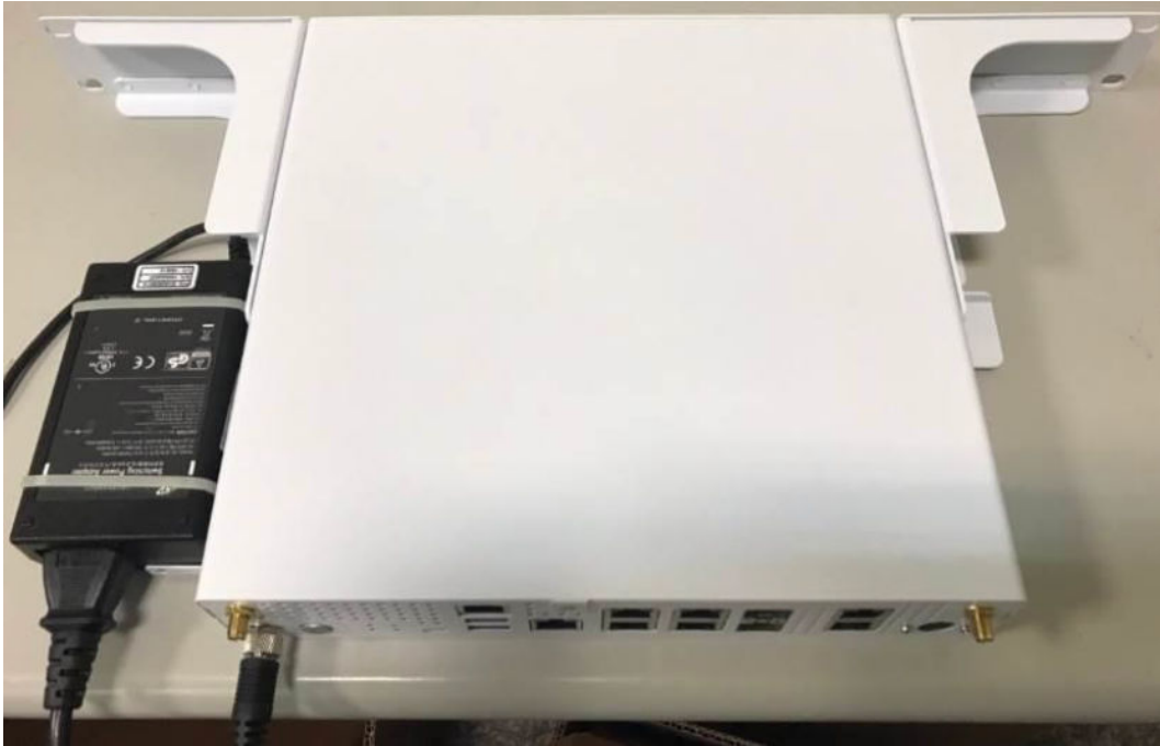
Figure 16: Assembled MicroVSP in Two-Post Mount
