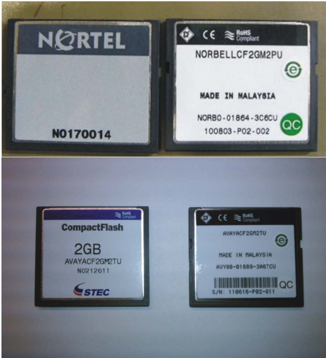
Figure 2. Front and rear view of good internal CF cards (without microcode errata)
