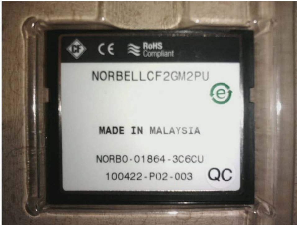
Figure 1. Suspect internal CF card (needs to be replaced)
