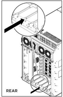
3. Before you fully insert the module into the slot, rotate the action levers away from the module until they form a 90° angle with the front of the module then carefully slide the module partway into the slot.
