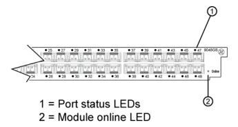
Figure 4: 9048GB module LEDs
