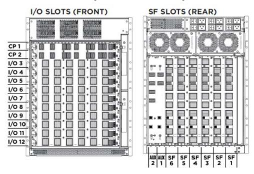
2. Align the module base-plate with the guide rails on either side of the opening for horizontal modules or the guide rails at the top and bottom of the opening for vertical modules.
