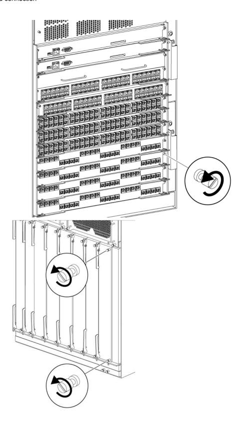
3. Rotate the insert or extract levers to eject the module from the chassis as shown in the following figures.
