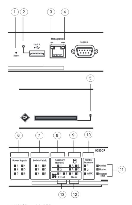
Figure 7: 9080CP module LEDs
