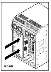
5. Continue seating the module by rotating the action levers until the levers are parallel with the front face panel and the module is fully seated.
