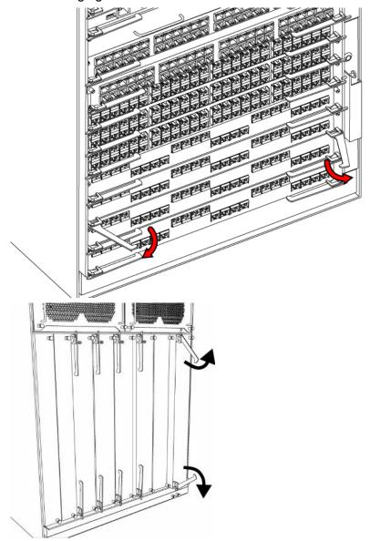
4. Slide the module out of the chassis as shown in the following figures.
