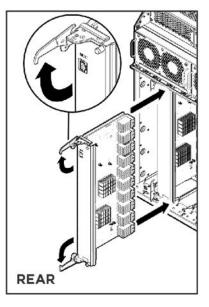
4. Apply equal force to each action lever to insert the module into the slot until the module stops moving. Gently seat the module interface connectors by pressing on the outside edges of the module near the action levers.
