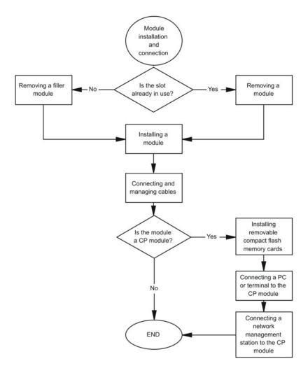
Figure 12: Module installation and connection procedures
