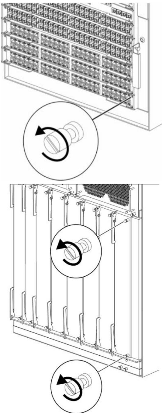
3. Rotate the insert or extract levers to eject the module from the chassis as shown in the following figures.
