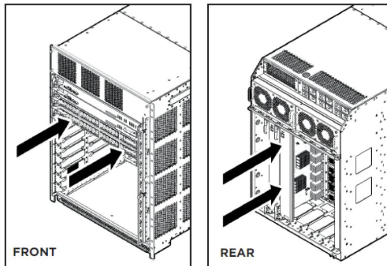
5. Continue seating the module by rotating the action levers until the levers are parallel with the front face panel and the module is fully seated.
