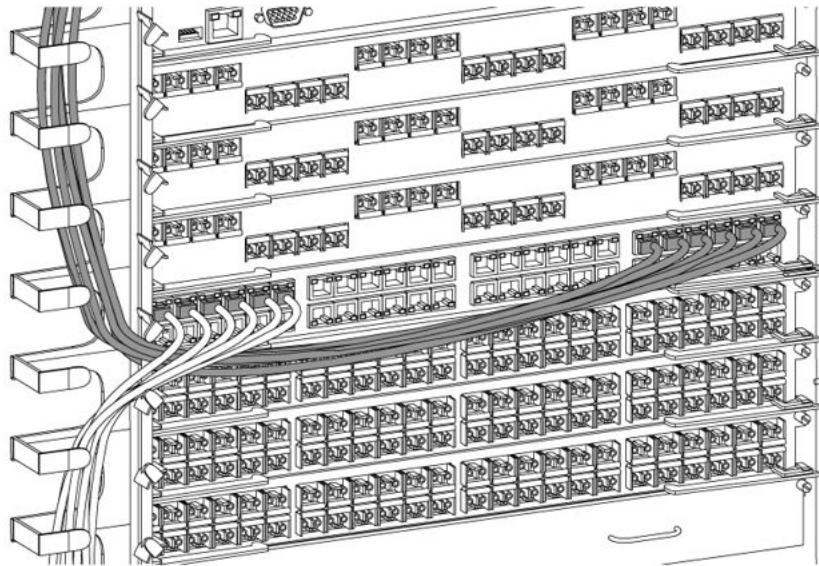
3. Route the cable to the termination panel, loosely fastening it with Velcro straps or sheet fiber along the path.
