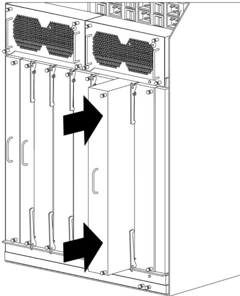
3. Use the two handles on the front filler module or the one handle on the back filler module to seat the module midplane connectors.
