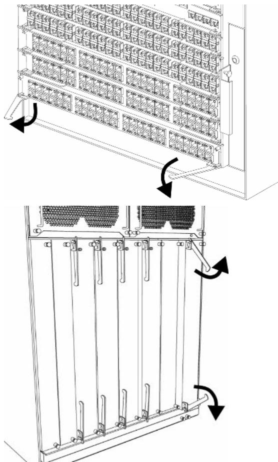
4. Slide the module out of the chassis as shown in the following figures.
