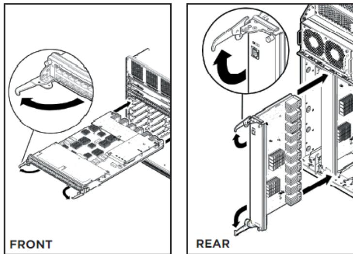
4. Apply equal force to each action lever to insert the module into the slot until the module stops moving. Gently seat the module interface connectors by pressing on the outside edges of the module near the action levers.
