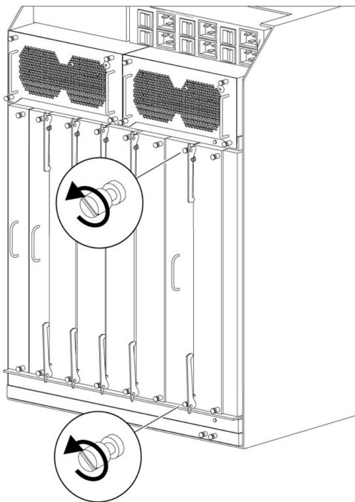
2. Grasp the two handles on the front filler module or the one handle on the back filler module.
