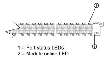
Figure 6: 9048GB module LEDs
