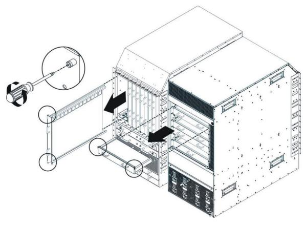
3. Pull the filler module away from the slot.
