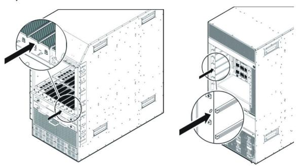
3. Before you fully insert the module into the slot, rotate the action levers away from the module until they form a 90° angle with the front of the module. Carefully slide the module partway into the slot.
