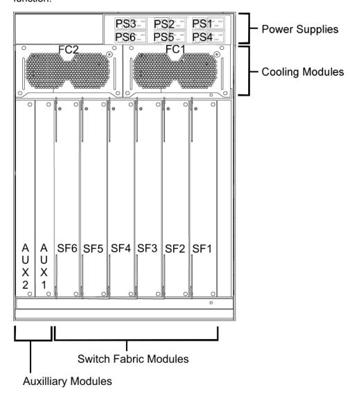
The SF module slots are numbered from right to left. The slot location determines the module function.
