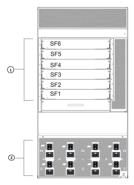
Figure 14: 9095SF module slot locations
