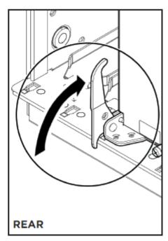
6. Turn both screws by hand until they catch, before you tighten the screws, which allows the module to move a little to catch the screws. Use a Phillips screwdriver to tighten the screws until snug. Do not overtighten. Do not use a power tool to tighten screws.
