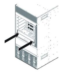
5. Continue seating the module by rotating the action levers until the levers are parallel with the front face panel and the module is fully seated.
