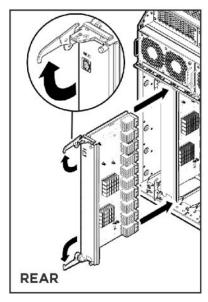
4. Gently seat the module interface connectors by pressing on the outside edges of the module near the action levers.
