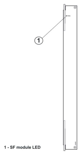
Each SF module connects to 10 I/O module slots and 2 CP module slots simultaneously. You can install a maximum of 6 SF modules in each chassis in an N + 1 configuration with redundancy.
