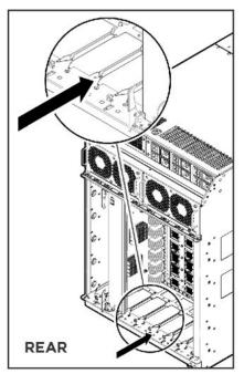
3. Before you fully insert the module into the slot, rotate the action levers away from the module until they form a 90° angle with the front of the module. Carefully slide the module partway into the slot.
