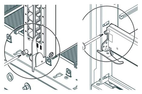
3. Rotate the insert or extract levers to eject the module from the Virtual Services Platform 9010.
