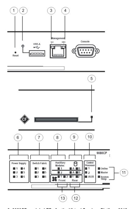
Figure 9: 9080CP module LEDs for the Virtual Services Platform 9012
