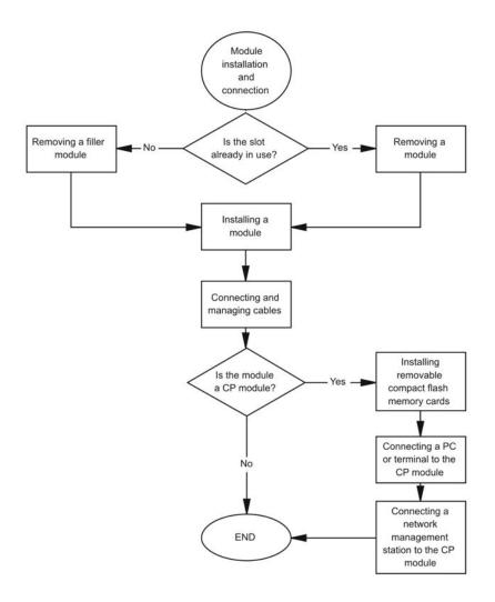
Figure 22: Module installation and connection procedures
