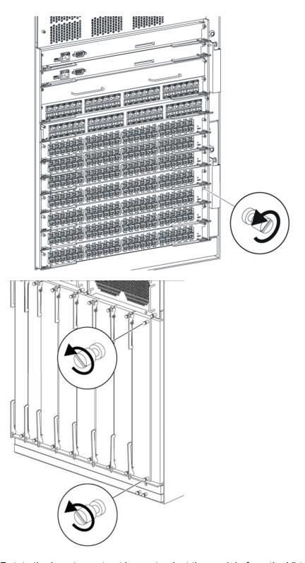
3. Rotate the insert or extract levers to eject the module from the Virtual Services Platform 9012 as shown in the following figures.
