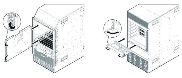
4. Gently seat the module interface connectors by pressing on the outside edges of the module near the action levers.
