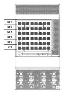
2. Align the module metal baseplate with the guide rails on either side of the opening for horizontal modules or the guide rails at the top and bottom of the opening for vertical modules.
