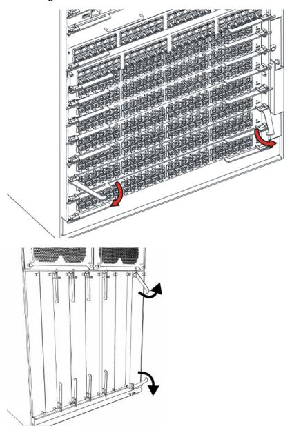
4. Slide the module out of the Virtual Services Platform 9012 as shown in the following figures.
