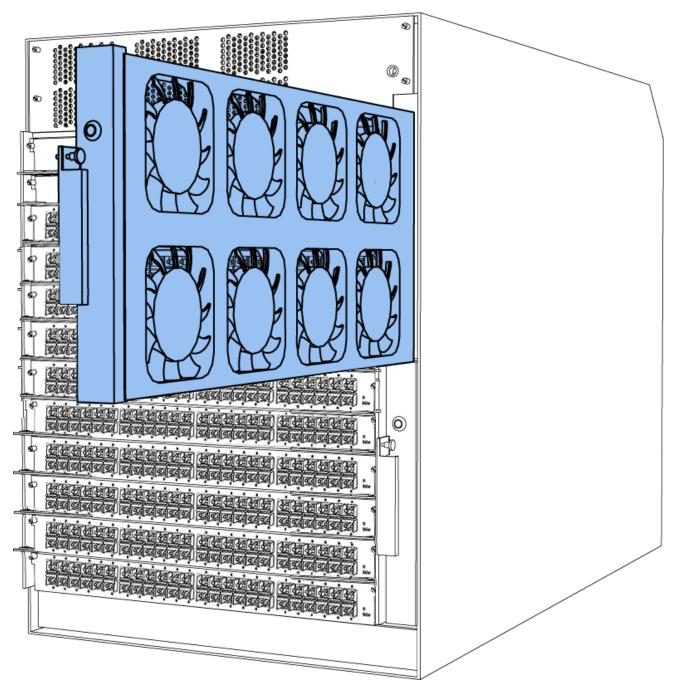
Figure 18: 9012 cooling module
