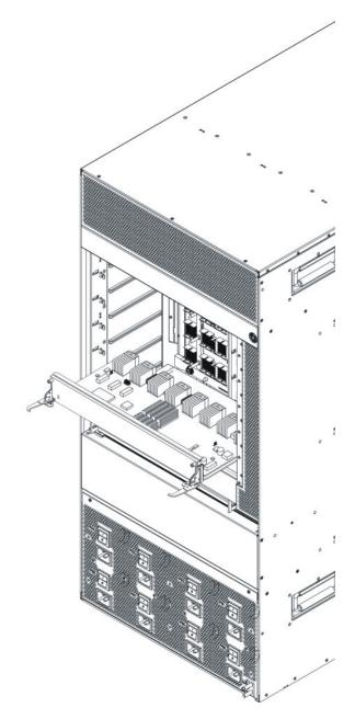
Do not operate a chassis without either a filler module or a module installed in a slot.
