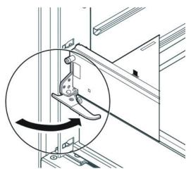
6. Turn both screws by hand until they catch, before you tighten the screws, which allows the module to move a little to catch the screws. Use a Phillips screwdriver to tighten the screws until snug. Do not overtighten. Do not use a power tool to tighten screws.
