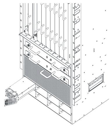
2. Rotate the action lever closed to seat the power supply and engage the retaining clip.
