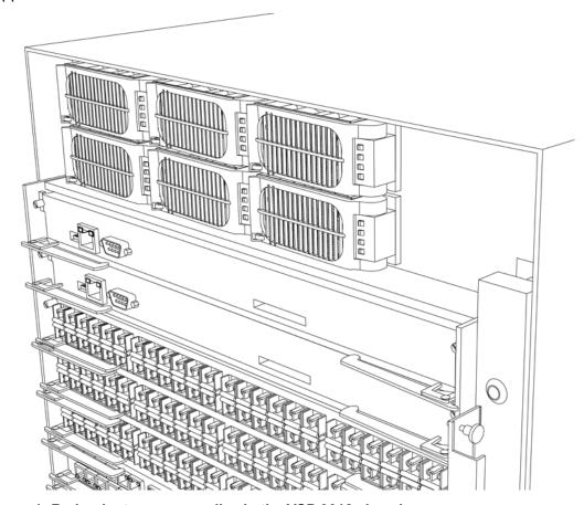
Figure 1: Redundant power supplies in the VSP 9012 chassis
