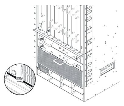
3. At the back of the chassis, connect an AC power cord from the AC power inlet to a power outlet.
