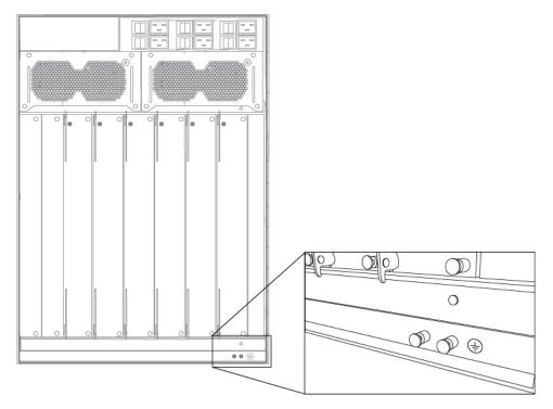
3. Bond the chassis ground cable to the single point ground window.
