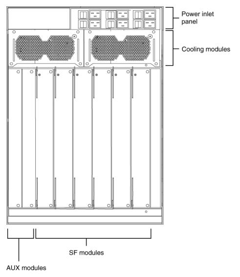
Figure 2: Virtual Services Platform 9000 chassis rear view
