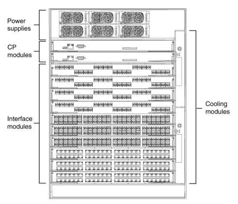
Figure 1: Virtual Services Platform 9000 chassis front view
