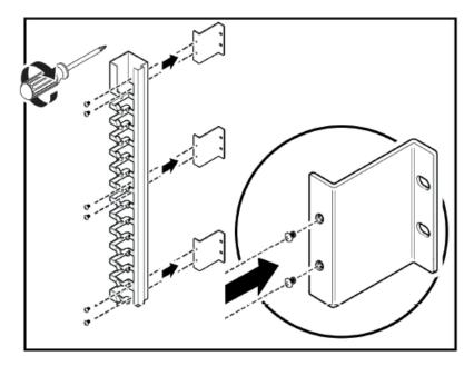
2. Use 3 Phillips screws to fasten the I/O cable management assembly to the top, middle and bottom screw positions of the left flange and rail.
