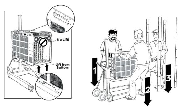
Use the recessed handles at the top and bottom of the chassis sides to lift the chassis. From the rear: Lift the chassis from the bottom only.
