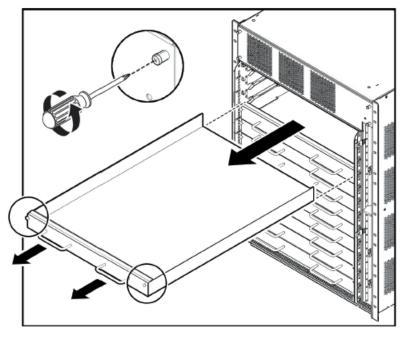
4. Remove the cooling modules by pulling the retaining pin that holds it in place while gently pulling the module's handle to move it out and away from the chassis.
