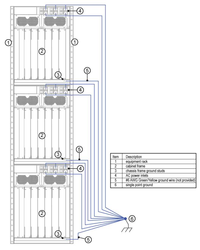
Figure 5: Rack grounding strip example
