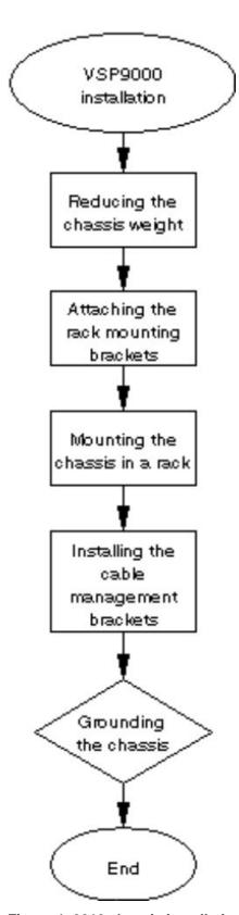
Figure 4: 9012 chassis installation procedures
