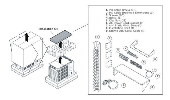
Figure 3: Accessories of the chassis shipping container
