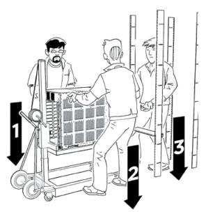
Use the recessed handles at the top and bottom of the chassis sides to lift the chassis. From the rear: Lift the chassis from the bottom only.
