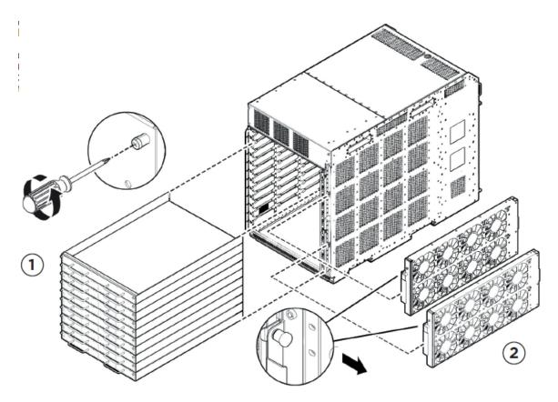
3. Unseat the I/O filler module by loosening the 2 captive screws, grasping the two handles, and gently pulling the module out and away from the chassis.
