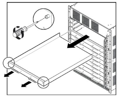
4. Remove the cooling modules by pulling the retaining pin that holds it in place while gently pulling the module's handle to move it out and away from the chassis.
