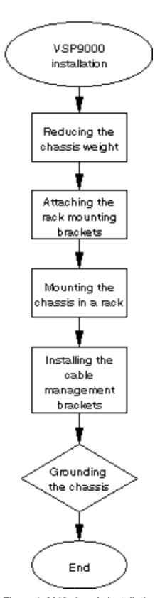
Figure 4: 9012 chassis installation procedures
