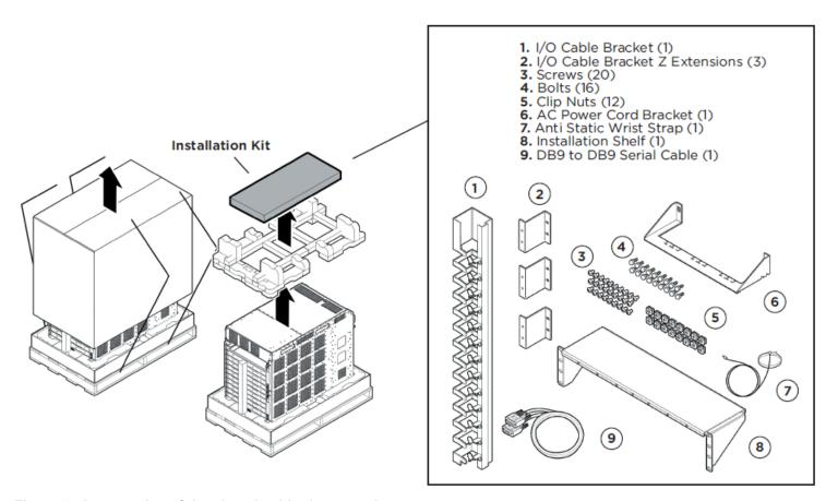
Figure 3: Accessories of the chassis shipping container
