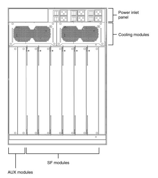
Figure 2: Virtual Services Platform 9000 chassis rear view
