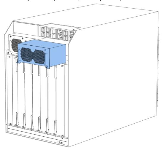
Figure 13: 9012RC cooling module
