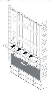
2. Use the screws to attach the bracket to the chassis.
