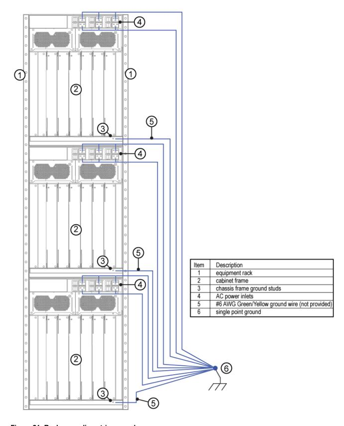
Figure 21: Rack grounding strip example
