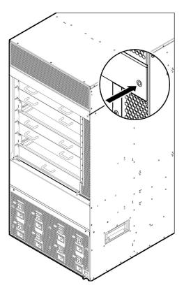
Figure 8: ESD ground strap input (rear)
