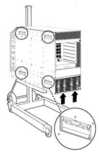
2. From the rear of the chassis, lift the chassis from the bottom only.
