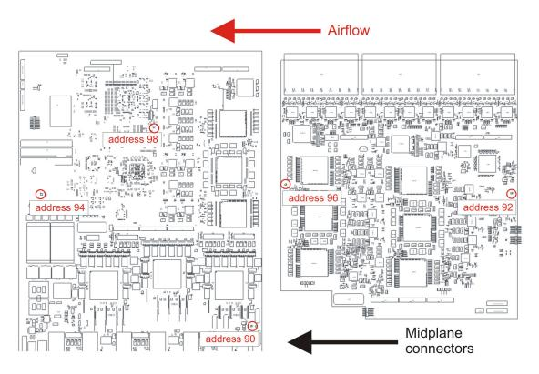
Figure 15: Heat sensor locations in a second generation I/O module
