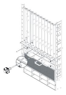
3. Align the hooks on the cover with the slots on the mounting bracket and with the keyholes on the chassis.
