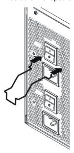
2. Push the L-shaped ends up to fully engage the retainer.
