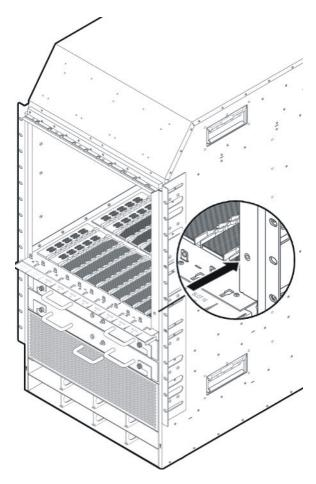
Figure 7: ESD ground strap input (front)
