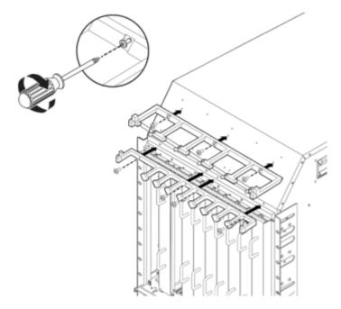
5. Align the tabs of each side of the cable management cover with the slots on the brackets.
