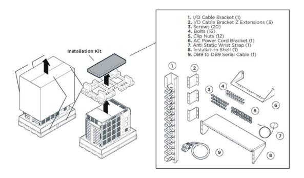
Figure 20: Accessories of the chassis shipping container
