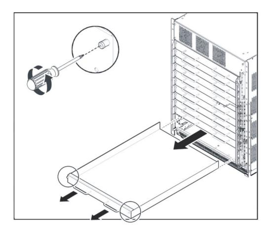
4. Remove the cooling modules by pulling the retaining pin that holds it in place while gently pulling the handle on the module to move it out and away from the chassis.
