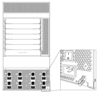
3. Bond the chassis ground cable to the single point ground window.
