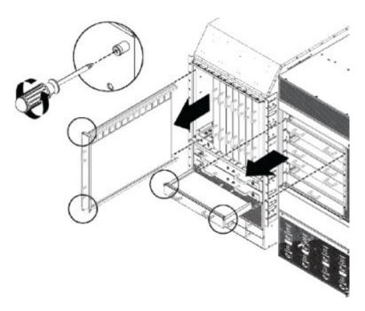
2. To unseat the cooling module, loosen the two captive screws, rotate the tabs to release the cooling module, and then grasp the two handles to gently pull the module out and away from the chassis.
