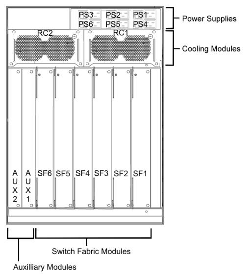
Figure 10: VSP 9012 chassis rear view
