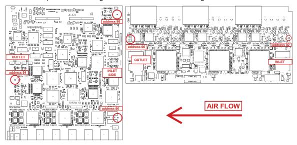
Figure 4: Heat sensor locations in a first generation I/O module
