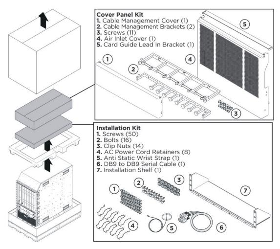
Figure 5: Accessories of the chassis shipping container
