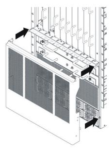
4. Insert the hooks into the slots and keyholes to secure the cover to the chassis.
