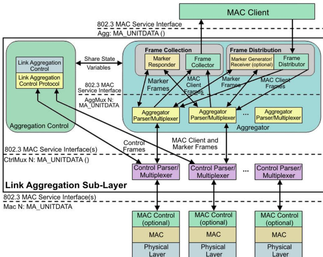
**Figure 1: Link aggregation sublayer (according to IEEE 802.3ad)**
