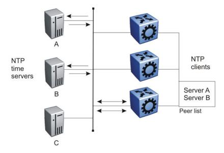
Figure 3: NTP time servers operating in unicast client mode
