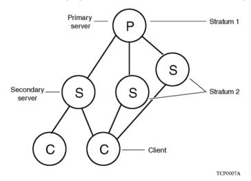
Figure 2: NTP time servers forming a synchronization subnet
