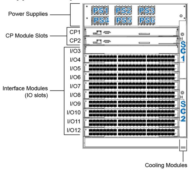
Figure 10: Virtual Services Platform 9012 front chassis slots
