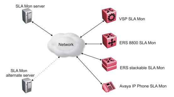
Figure 4: SLA Monitor network
