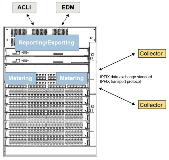
Figure 1: IPFIX collecting and reporting functions for first generation I/O modules
