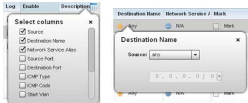
**Figure 6-21** IP Firewall Rules Add Criteria screen
