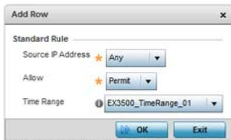
**Figure 10-22** EX3500 ACL Standard - Add Standard Rule screen
