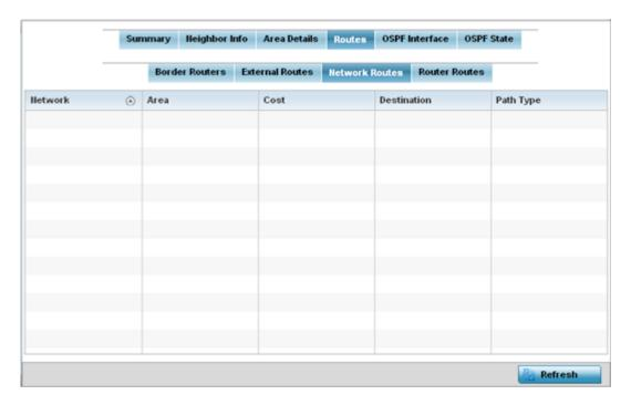
Network routes support more than two routers, with the capability of addressing a single physical message to all attached routers (broadcast). Neighboring routers are discovered dynamically using OSPF hello messages. This use of the hello protocol takes advantage of broadcast capability. An OSPF network route makes further use of multicast capabilities, if they exist. Each pair of routers on the network is assumed to communicate directly.
