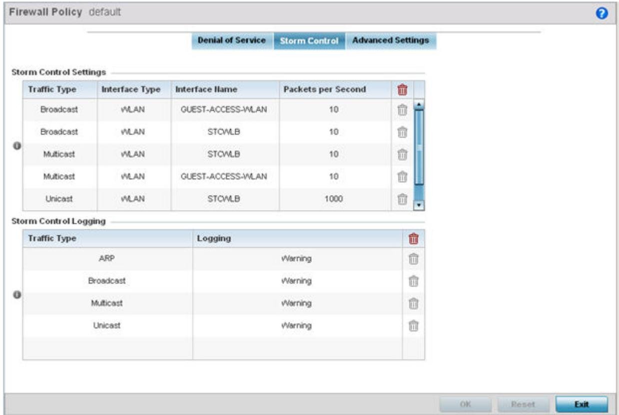
**Figure 344: Wireless Firewall - Add/Edit - Storm Control Screen**
