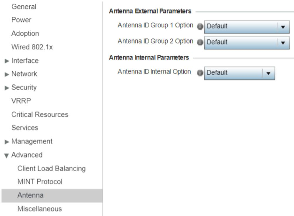
**Figure 125: Advanced Profile Overrides - Antenna Screen**
