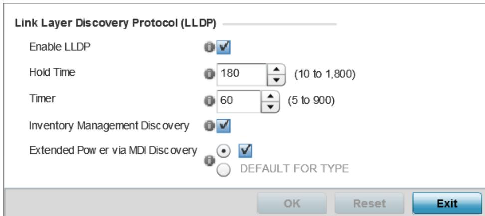
**Figure 208: Profile Overrides - Network - LLDP Configuration Screen**
