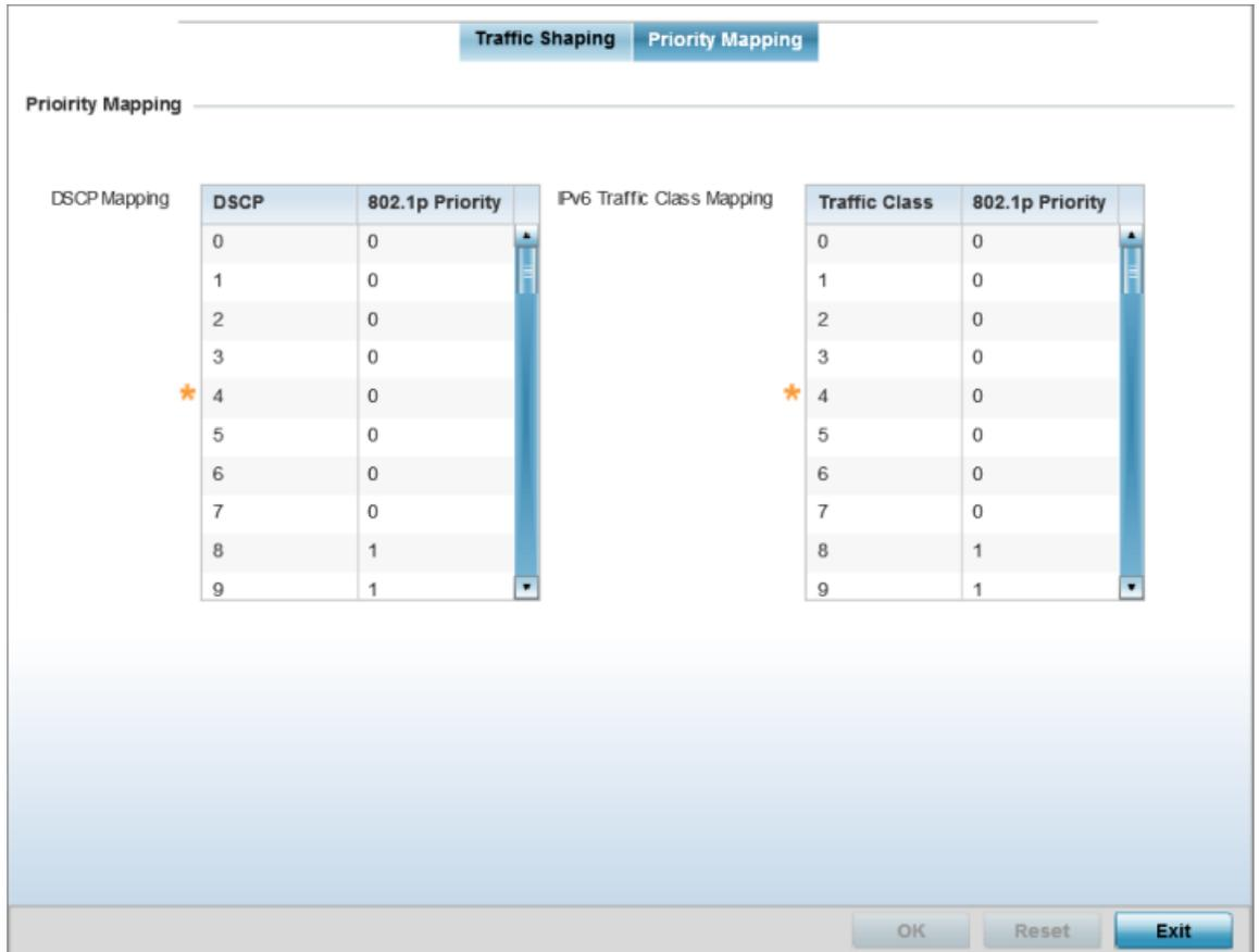
**Figure 53: QoS - Priority Mapping Configuration Screen**
