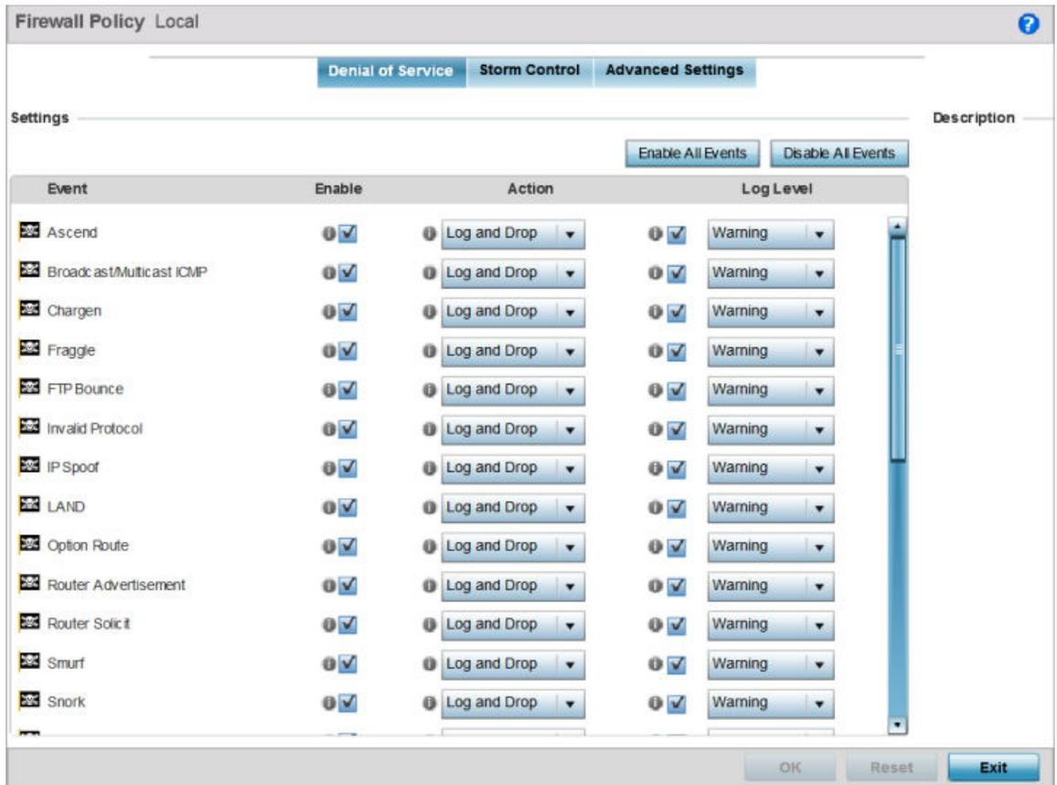
**Figure 343: Wireless Firewall Screen - Denial of Service Tab**
