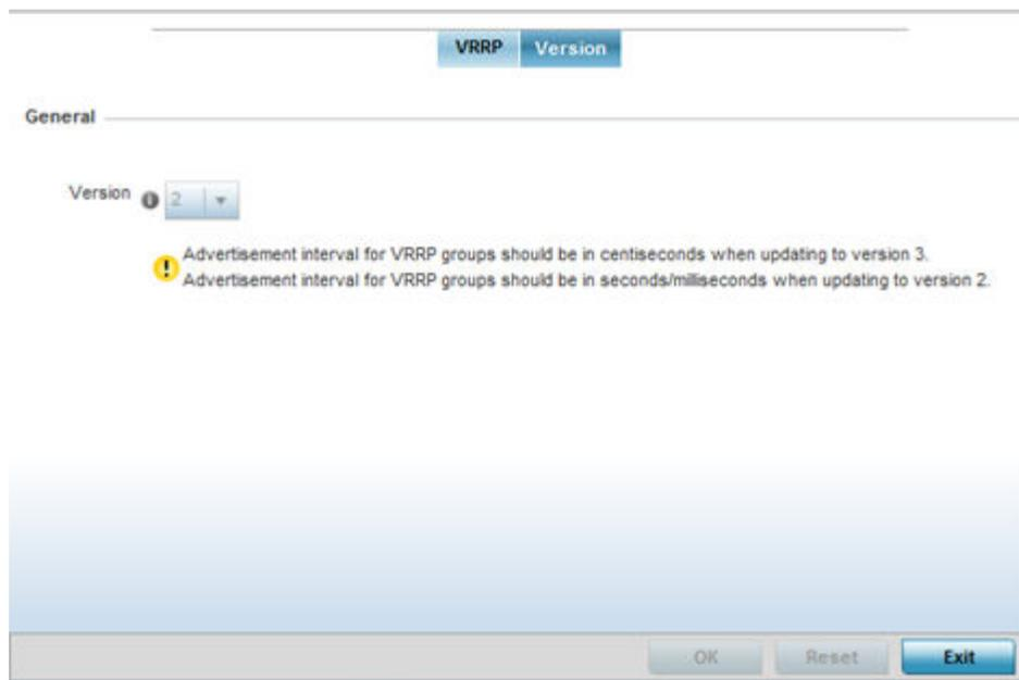
**Figure 241: Device Overrides - VRRP Screen - Version Tab**
