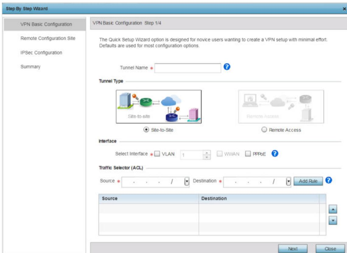
**Figure 219: VPN Basic Configuration Screen Step 1/4**
