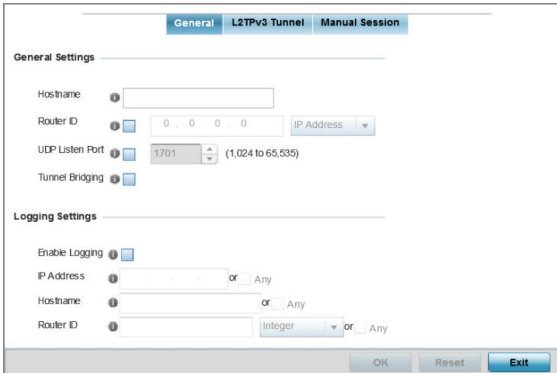
**Figure 46: Network - L2TPv3 screen - General tab**
