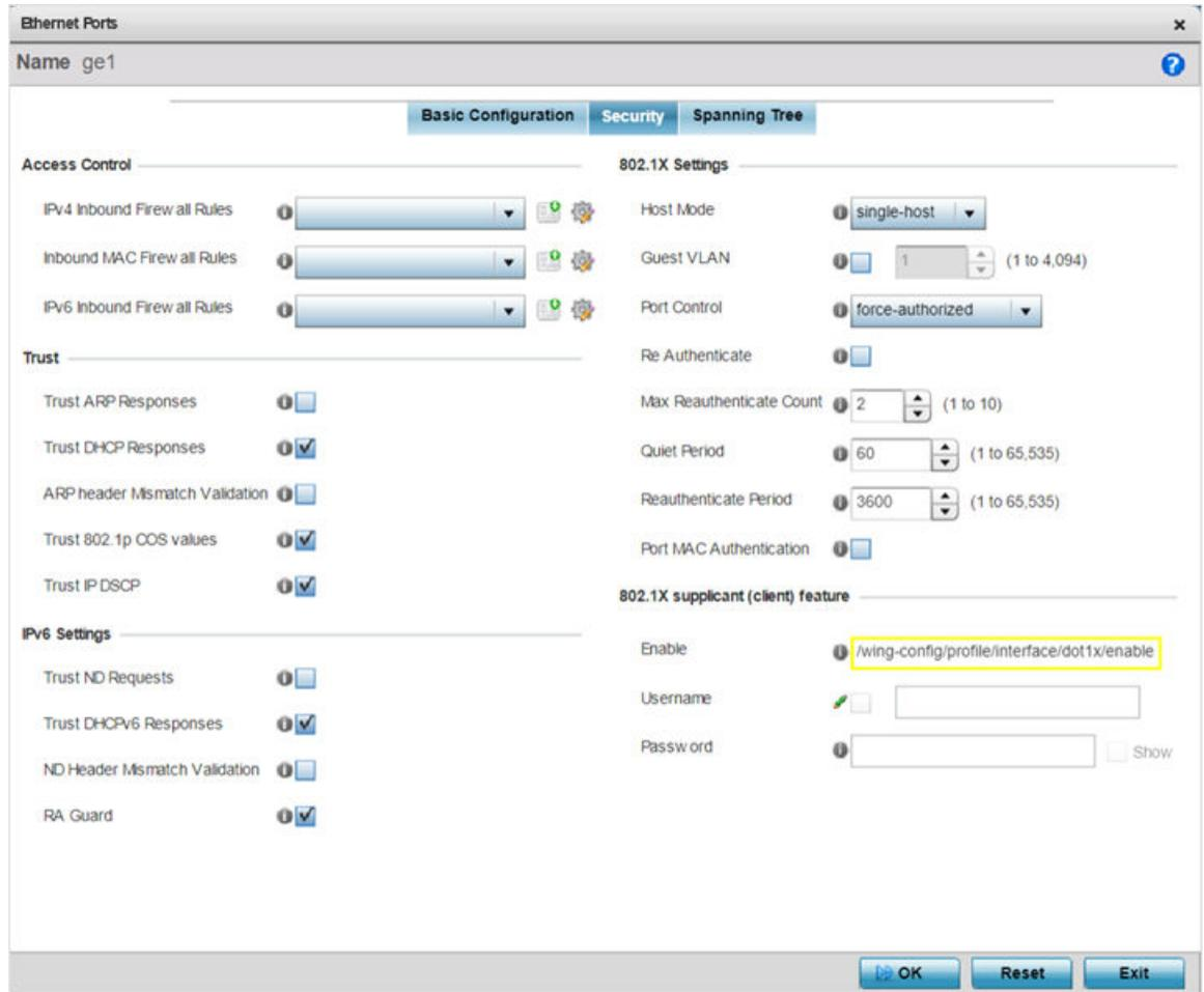
**Figure 27: Interface GE Port - Security Tab**
