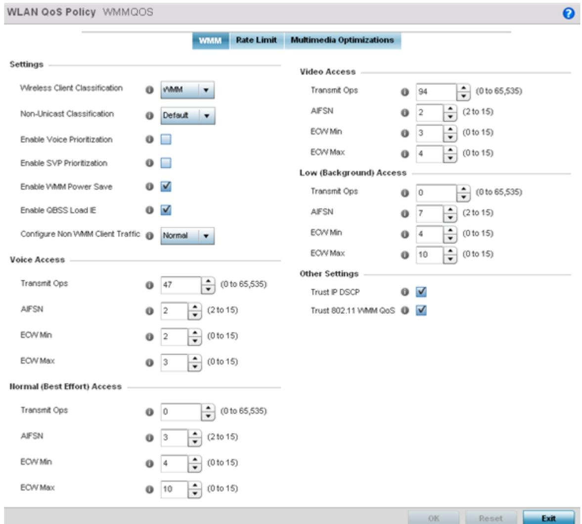
**Figure 304: WLAN QoS Policy Screen - WMM Tab**
