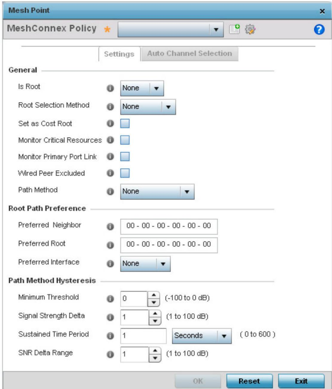
**Figure 112: Mesh Point Settings Screen**
