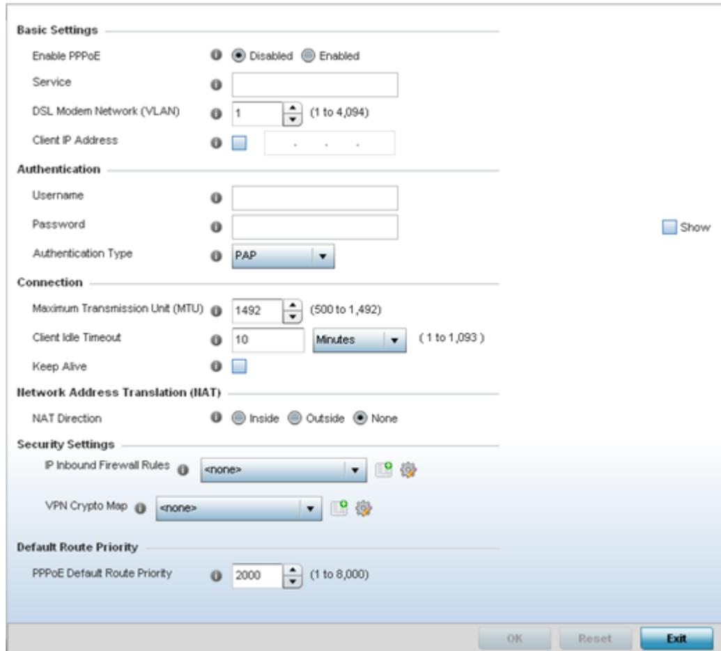
**Figure 170: Profile Overrides - PPPoE Interface Configuration Screen**
