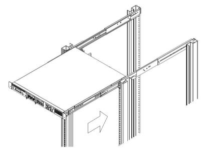
6 When the front of the unit is flush against the rack, securely attach the unit using the two M3 screws supplied with the kit.
