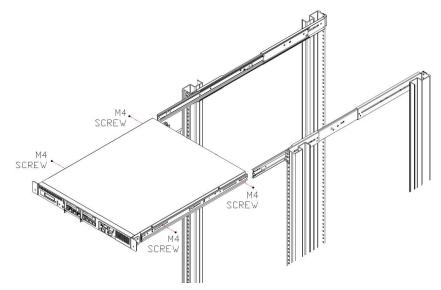
5 Align the inner and outer slide rails and carefully insert the unit into the rack.
