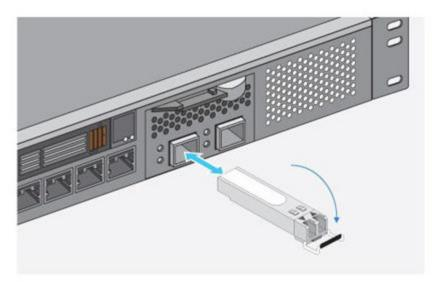
2 Press the transceiver into the slot until it clicks into place.
