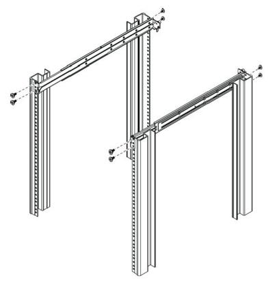
4 Using the four M4 screws supplied with the kit, attach the inner slide rails to the sides of the unit.
