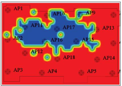
This visualization gives a general idea of the coverage for Wi-Fi Position Tracking and the values set above are assuming a larger deployment. If it is a smaller deployment, the "Infrastructure Service Count" may need to be decreased.
