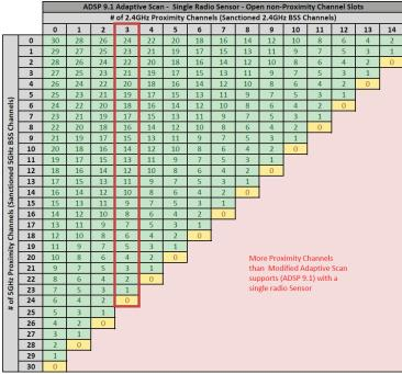
determine Proximity channel combinations. It should be noted that the more Proximity channels (Sanctioned BSS Channels) there are fewer time slots are available to rotate non-Proximity channels through. A value of '0' in the table means that there are no free slots to rotate in non-Proximity channels.
