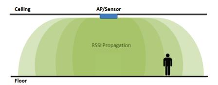
The following diagram illustrates distorted correlation of RSSI vs distance, for an AP at 30 feet ceiling height, with standard dipole antenna.
