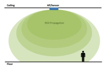
The following diagram illustrates positive correlation of RSSI vs distance, for an AP at 30 feet ceiling height, with external narrow beam panel antenna.
