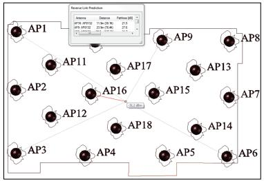
The Service Count and Instant Point predictions should be performed for each group of APs on the same channel that was determined with the manual channel layout. The overall design will be ready once all predictions show compliance with the Wi-Fi Position Tracking requirements. Typically, the AP density will come out to about an AP every 2500 square feet.
