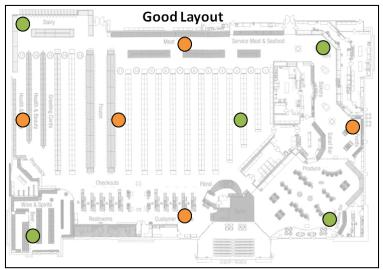
A general step by step method is to place sensors around the perimeter. Once the perimeter is configured, place sensors in the center. Finally, fill in the gaps between the perimeter and center to complete coverage.
