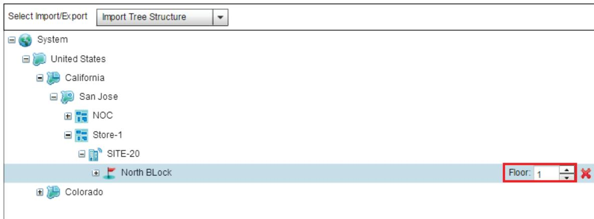
11. Move Access points on to the floor using drag & drop on NSight UI. Navigate to Map View -> Select RF-Domain -> Select Area: Floor:
