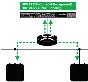
In a Centralized deployment IP based MINT links are used for clustering, the adoption and management of Site Controllers and Access Points (APs) and encapsulating Wi-Fi user traffic between Site Controllers and APs if tunneling has been enabled in one or more Wireless LANs. IP based MINT links are also used to encapsulate Wi-Fi user traffic from an elected RF Domain Manager (RFDM) at a remote site to the Centralized Controllers when tunneling over Level 2 MINT links is enabled.
