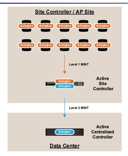
Once the Level 2 MINT links have been established, each remote Site Controller is assigned a Profile and RF Domain and its configuration is applied. The Site Controllers will then establish the cluster and elect an RF Domain Manager (RFDM) for the site. All but the elected RFDM would transition their Level 2 MINT links into an un-used state.
