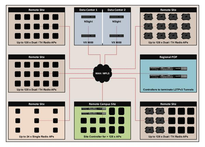
The centralized model can be scaled to support up to 10,240 remote sites and as of WING 5.5 each remote site can support up to 128 x Dual or Tri Radio Access Points or 24 x Single Radio Access Points. For sites with more than 128 x Access Points, site controller can be deployed to account for AP capacity of the site.
