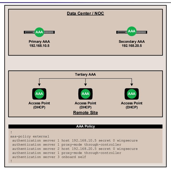
When backup RADIUS services are provided locally on the Independent Access Points at a site, a RADIUS Server Policy will need to be defined and assigned to the Access Point Profile. The RADIUS Server Policy includes the RADIUS Server configuration along with specific User Pools. During a WAN outage, each Independent Access Point will be fully capable of authenticating EAP or Hotspot users locally providing no interruption to Wireless services at the remote site.
