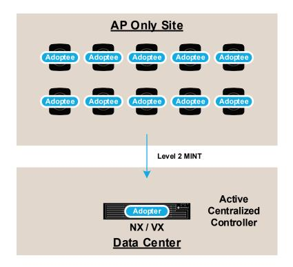
Once the Level 2 MINT link has been established, the remote APs are assigned their Profile and RF Domain and their configuration applied. The APs then discover all the other APs at the site via the Control-VLAN and elect an RF Domain Manager (RFDM) for the site. All but the elected RFDM will transition their Level 2 MINT links into an un-used state.
