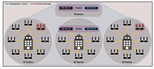
Each elected RFDM maintains the IP based Level 2 MINT link to the Active Centralized Controller in the data center. The Level 2 MINT link is used to forward all the MINT management / control traffic and encapsulated user traffic exchanged between the data center and remote site. The RFDM also has additional responsibilities within the RF Domain which includes:
