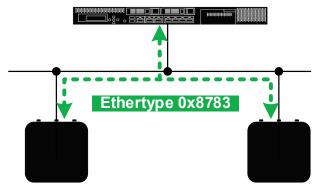
In a Centralized deployment VLAN based MINT links used in Access Point (AP) only sites to allow the APs at a site to discover themselves and elect an RF Domain Manager (RFDM) for the site. The VLAN based MINT links are automatically established by defining a Control-VLAN to each RF Domain for the AP only sites.
