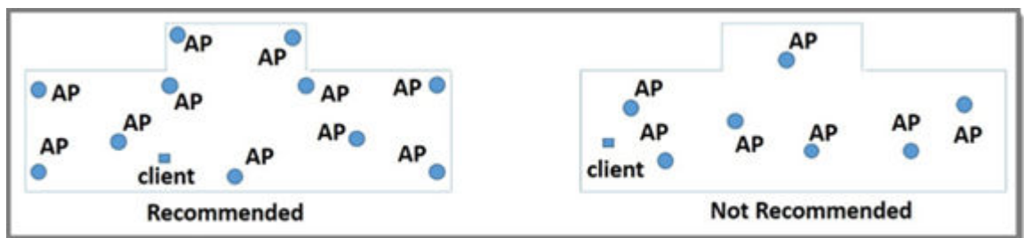
Figure 4: Recommended AP Placement
