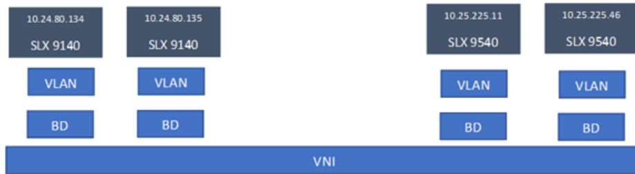
Figure 18: Scope of tenant constructs
