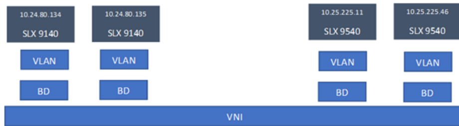
Figure 17: Scope of tenant constructs
