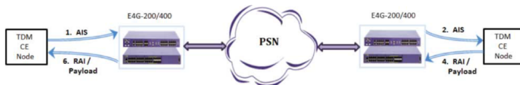
Figure 22: SAToP Alarm Handling: TDM Service AIS Alarm
