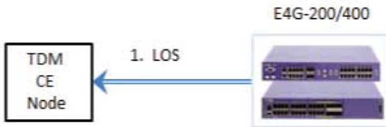
Figure 16: LOS Alarm Generation
