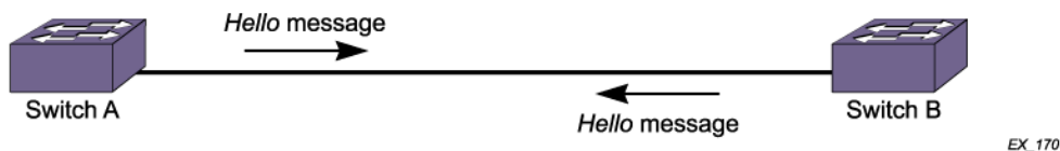
Figure 61: Extreme Networks Switches with ELSM-Enabled Ports Exchanging Hello Messages
