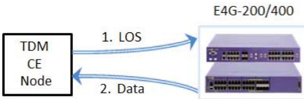
Figure 17: LOS Alarm Response
