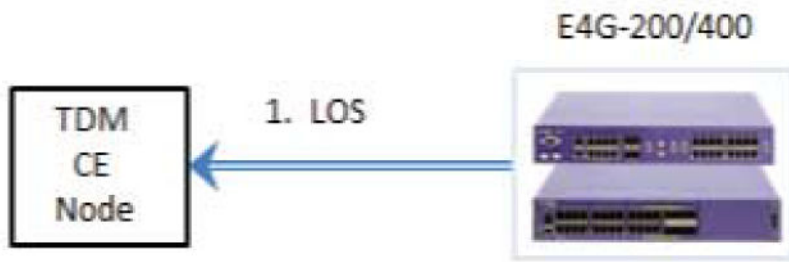
Figure 20: LOS Alarm Generation
