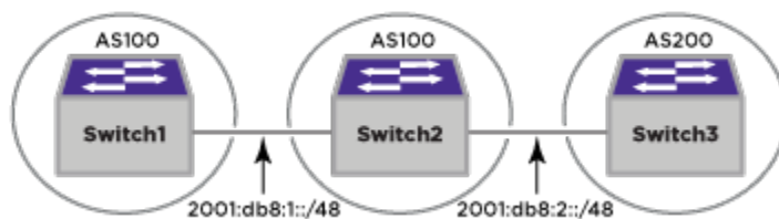
Figure 265: BGP IPv6 Example
