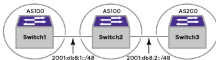
Figure 264: BGP IPv6 Example
