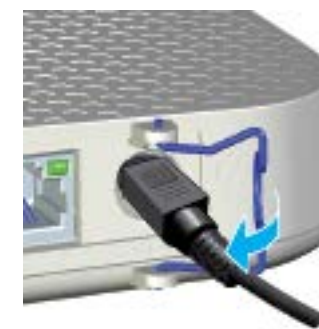
Figure 7 Power cable retainer
