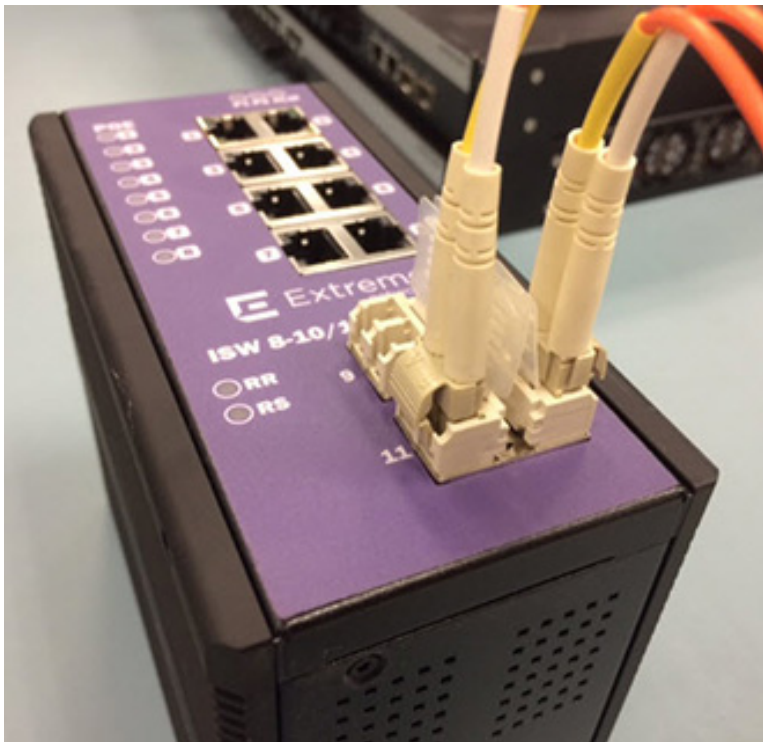
Figure 7: Connect the optical fiber to the SFP socket
