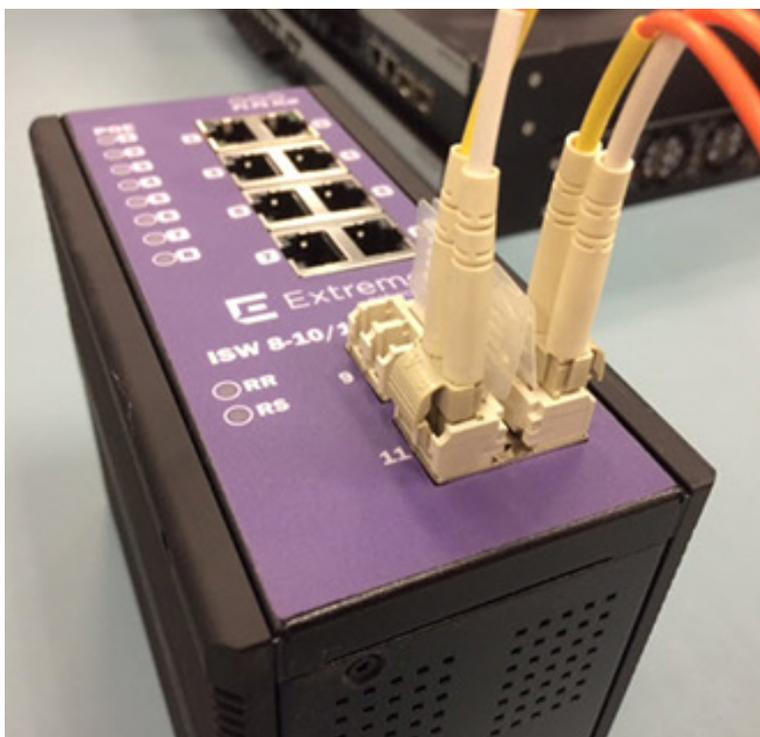
**Figure 8: Connect the optical fiber to the SFP socket**
