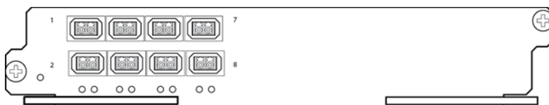
FIGURE 16 NI-MLX-10Gx8-M and NI-MLX-10Gx8-D module faceplate
