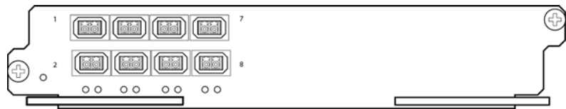
FIGURE 13 8x10GE-X module faceplate
