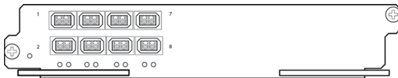
FIGURE 13 8x10GE-X module faceplate
