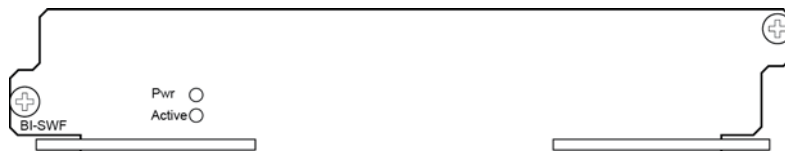
FIGURE 25 Switch fabric module front panel
