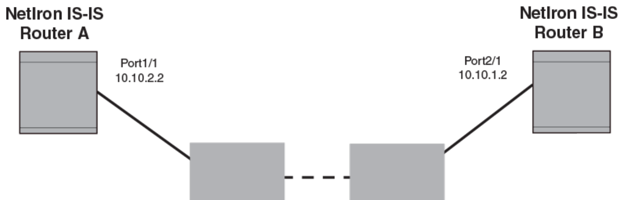
FIGURE 40 IS-IS Point-to-Point configuration
