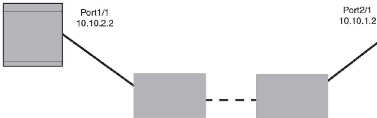
Figure 45: IS-IS Point-to-Point configuration
