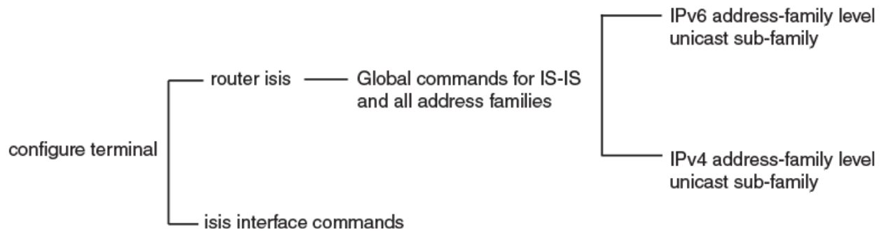
FIGURE 48 IPv6 IS-IS CLI levels
