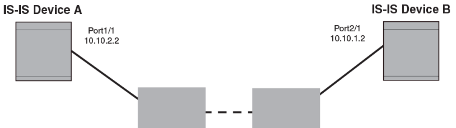
FIGURE 45 IS-IS Point-to-Point configuration
