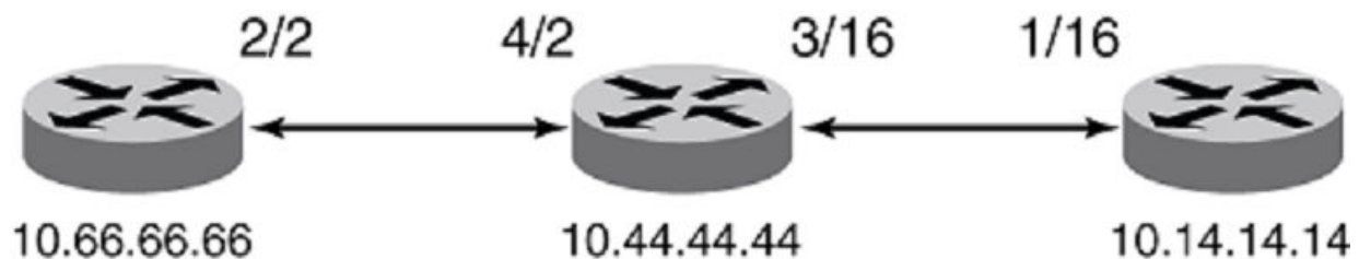
FIGURE 50 Inbound FEC filtering example
