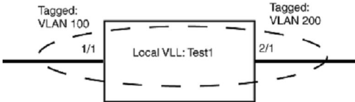
FIGURE 70 Local VLL "Test1" with two tagged VLANs
