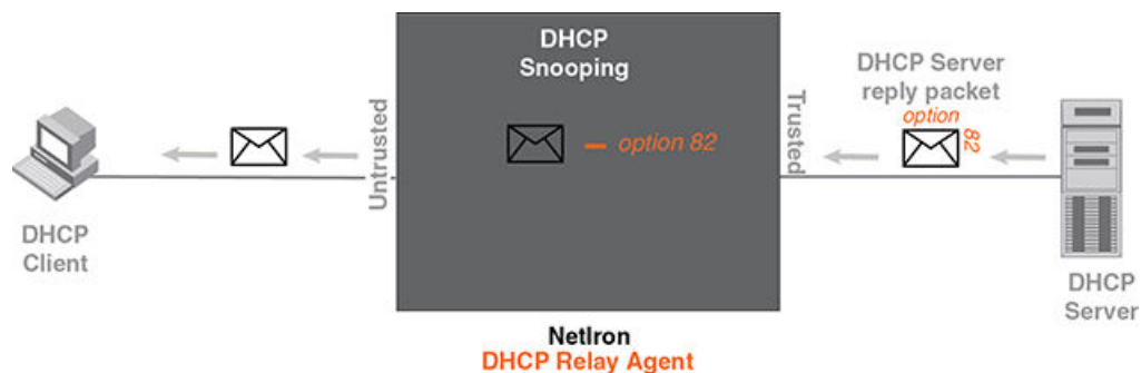
FIGURE 39 DHCP option 82 is removed from the packet
