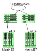
The figure above shows a common configuration in which a routed backbone is using both RIP and OSPF for its routing protocols. The network administrator does not want the multicast OSPF and broadcast RIP frames propagated to the end stations. The network is designed so that only end users are attached to the E7 devices.
