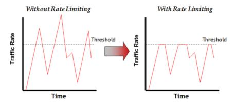
The CoS can be configured to perform one or all of the following actions when a rate limit is exceeded:
