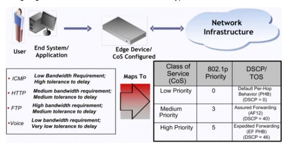
The ICMP protocol, used for error messaging, has a low bandwidth requirement, with a high tolerance for delay and jitter, and is appropriate for a low priority setting. HTTP and FTP protocols, used respectively for browser-generated and file transfer traffic, have a medium to high bandwidth requirement, with a medium to high tolerance for delay and jitter, and are appropriate for a medium priority level. Voice (VoIP), used for voice calls,
