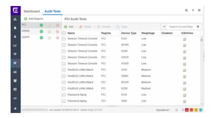
The Audit Test list contains a list of all of the audit tests available in Extreme Management Center, contained within the regulatory and standards regime of which it is a part. Each individual audit test displays the device types on which the test can be run in the **Device Type** column.
