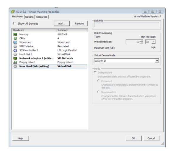
Repeating these steps to add additional drives results in different labels for those drives. For example, the label on the first drive you add is /dev/sdb, while the next drive added is labeled /dev/sdc.
