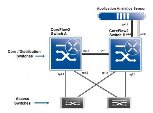
The servers in this network are connected to the ToR switches and must traverse core switches Switch A and Switch B to reach their clients. It is assumed that spanning tree will keep a loop-free topology and no load traffic balancing algorithms are run in the interfaces between the ToR/EoR switches and Switch A and Switch B.
