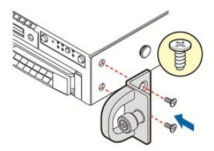
Installing the Rack Handles
