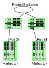
The figure above shows a common configuration in which a routed backbone is using both RIP and OSPF for its routing protocols. The network administrator does not want the multicast
