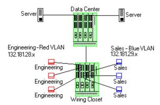
The figure above shows a configuration where the network administrator wants to separate end-user traffic into VLANs based on the assigned IP subnet of each department. This can easily be accomplished by creating two Layer 3 classification rules based on the IP subnet range of the respective departments.
