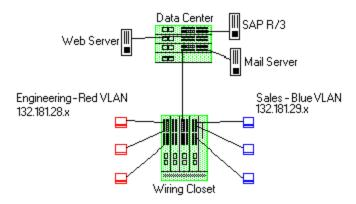
To accomplish the prioritization goals in this example, there are two main steps required: creating the classification rules, and then configuring the priority-to-transmit queue mapping for the switch, if needed.
