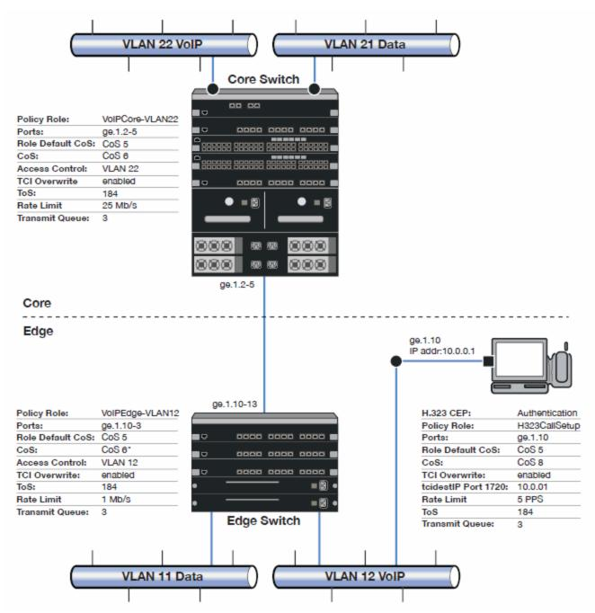
Edge and Core port groups in the RTP/Voice/Video (Static) CoS provide for the difference in rate limiting needs between the end user and aggregation devices. A VoIP Call Setup CoS provides rate limiting for the setup aspect of the VoIP call.
