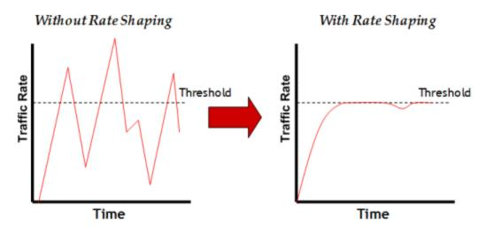
Rate shaping retains excess packets in a queue and then schedules these packets for later transmission over time. Therefore, the packet output rate is smoothed and bursts in transmission are not propagated as seen with rate limiting.
