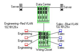
The figure above shows a configuration where the network administrator wants to separate end-user traffic into VLANs based on the assigned IP subnet of each department. This can easily be accomplished by creating two Layer 3 classification rules based on the IP subnet range of the respective departments.
