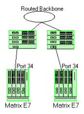
The figure above shows a common configuration in which a routed backbone is using both RIP and OSPF for its routing protocols. The network administrator does not want the multicast
