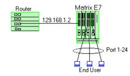
In the figure above, the network components include a router and an E7 device. In this configuration end-users connect to the ports of the E7 device.
