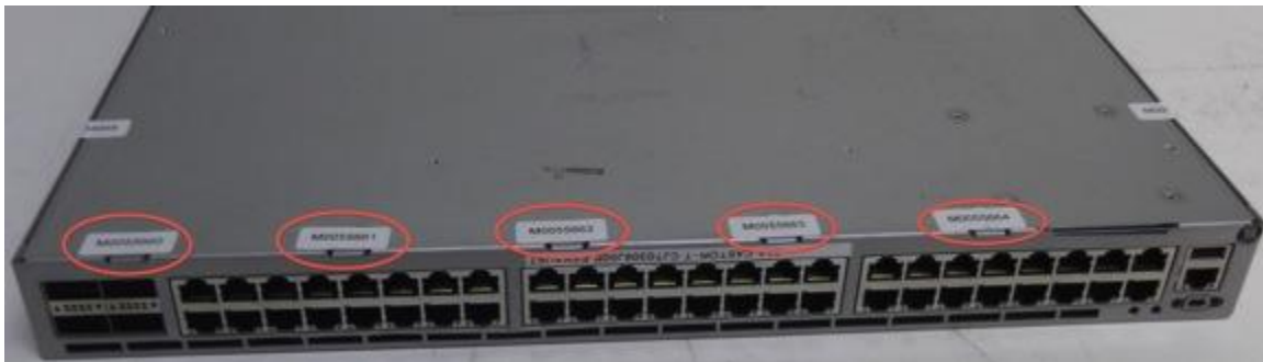
Figure 6. Brocade VDX 6740T bottom port-side seal locations
