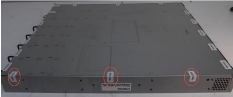
Figure 8 Brocade VDX 6740T bottom right-side seal locations
