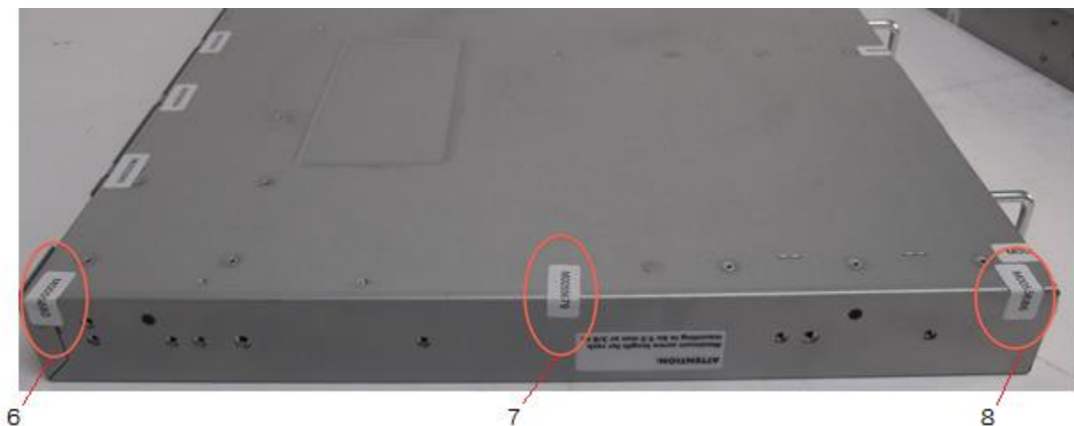
Figure 2. Brocade VDX 6740 bottom left-side seal locations
