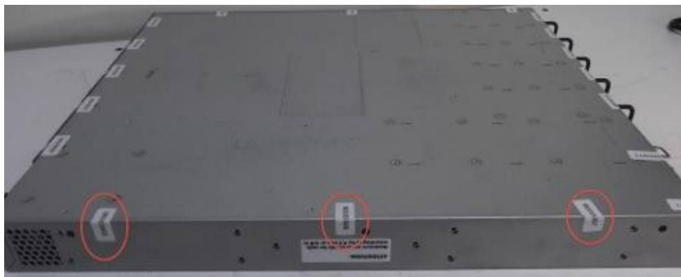
Figure 7. Brocade VDX 6740T bottom left-side seal locations
