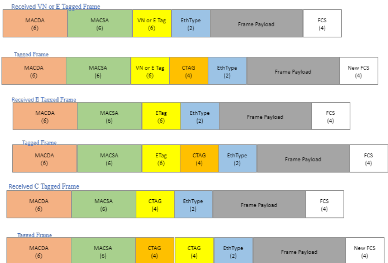
Figure 7: Tag addition, E-tag, VN-tag and C-tag frames
