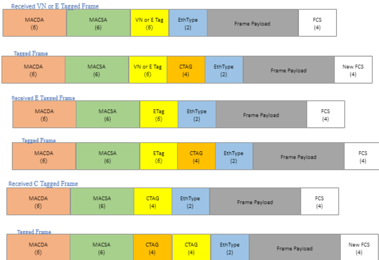
Figure 8: Tag addition, E-tag, VN-tag and C-tag frames
