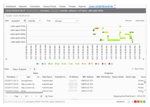
The RSS graph at the top of the tab shows the signal strength (in dBm) between the end-point and each of the APs to which it connected. The shape of the endpoint event indicators in the graph indicate the type of event.
